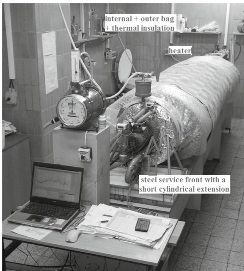
**Figure 2.** Fermentation bag used for the laboratory test
