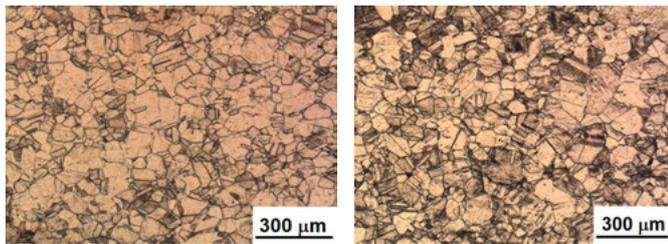
c) sample after the 4<sup>th</sup> pass      d) sample after the 6<sup>th</sup> pass
