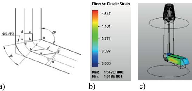
Fig. 1. a) Principle of the ECAP, where  $\Phi$  is the angle of transition of two channels and  $\Psi$  curvature of transition, b) FEM strain simulation for Al alloy (after the 1<sup>st</sup> pass through the ECAP tool)
