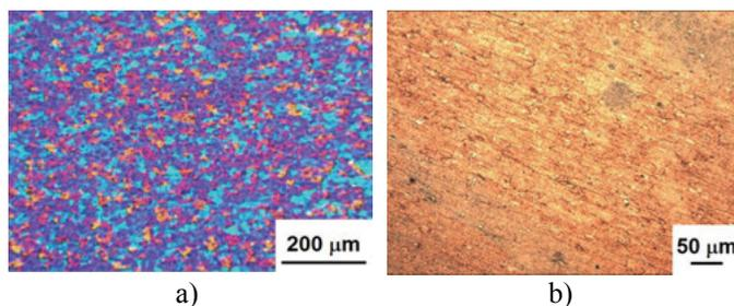
Fig. 6. Microstructure of the AlMn1Cu alloy a) initial state, b) after the 6<sup>th</sup> pass
