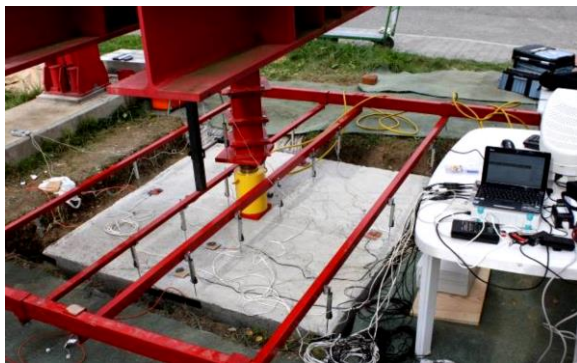
Fig. 2 Load test of the steel-fibre concrete slab
