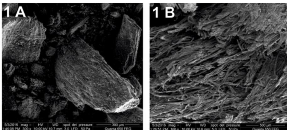
Fig. 1 Examples of pyrolytic products: A – biochar of wood, B – char of TetraPak from SEM microscope
