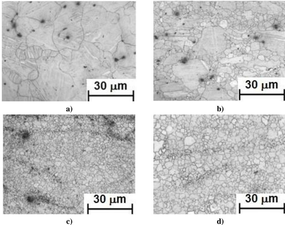
**Fig. 3** LOM - microstructure of AZ31: a) initial state -hot extruded (EX), b) one ECAP pass, c) third ECAP pass, d) fourth ECAP pass
