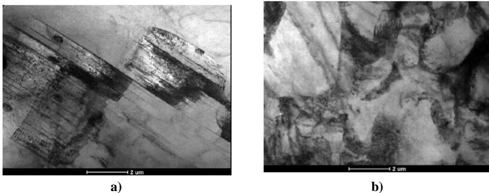
**Fig. 4** TEM micrographs of AZ31: a) a) initial state -hot extruded (EX), b) fourth pass
