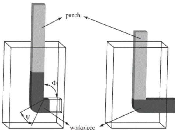
**Fig. 1** The principle of Equal Channel Angular Pressing (ECAP) method [3]
