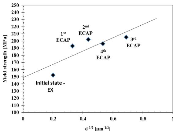
**Fig. 5** Hall – Petch relationship for AZ31 processed by hot extrusion and ECAP
