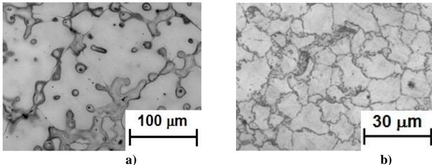
**Fig. 2** Structure of AZ31: a) as – casted state, b) hot extruded (EX) [6]
