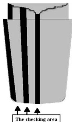
**Figure 1:** Layout of samples for analyses of the chemical composition
