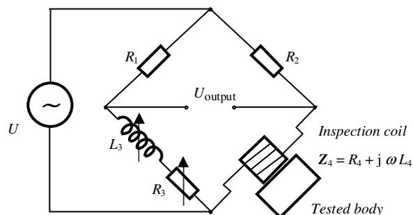
Fig. 2. AC bridge for ECT signal measurement.
