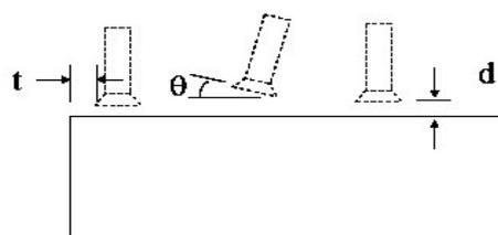
Fig. 4. Positions of ECT probes above tested object.
