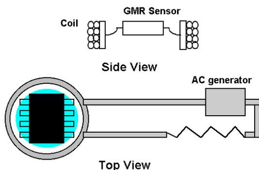
Fig. 5. Setup of ECT with GMR sensor.
