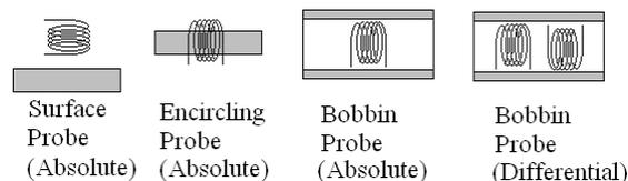
Fig. 3. Configurations of ECT Probes.
