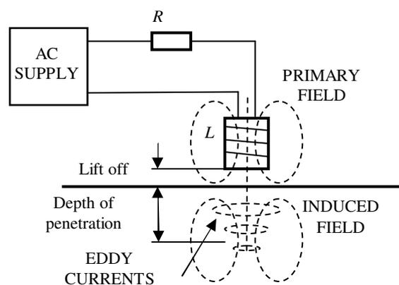
Fig. 1. Eddy current testing arrangement.
