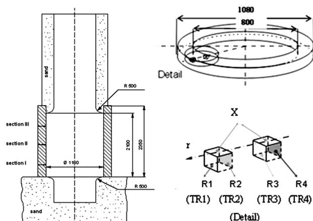
**Figure 1:** The set-up of a vertically cast roller and sampling
