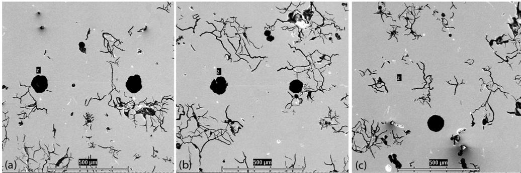
**Figure 2:** The structures in the area of sample TR1 selected for analysis: a) between two spheres of graphite through perlite, b) between the two spheres of graphite through cementite, c) through lamellar graphite
