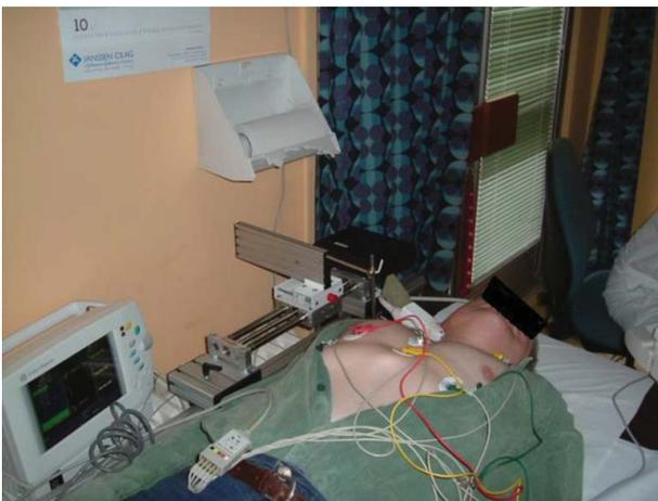
Figure 4. Configuration of the proposed device for the 3D ultrasound display and measurement of the atherosclerotic plaque.
