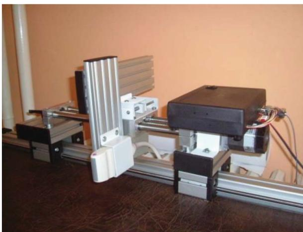
Figure 1. Positioning mechanism of the ultrasound probe.
