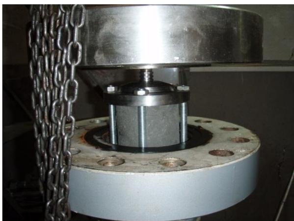
**Fig. 7.** Sample installation inside the pressure chamber with the testing container connected to the RK-2 lid by pressure line
