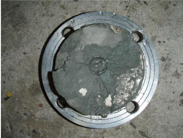
**Fig. 9.** Horizontal-vertical crack rock sample from the borehole H 111 after test of fracturing
