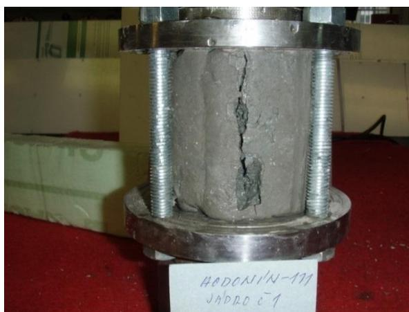
**Fig. 8.** Rock sample cored in H 11 after the laboratory fracturing experiment – on the front face of the sample is apparent vertical fracture
