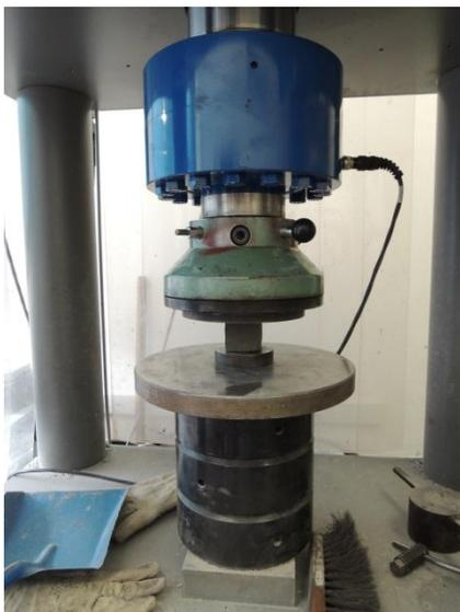
**Fig. 5.** Apparatus for evaluation of compressive strength
