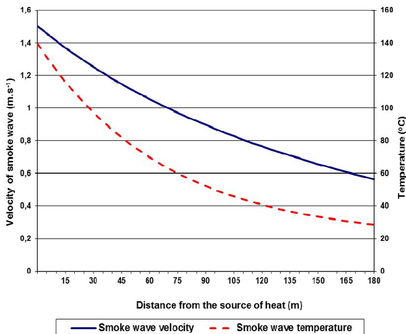
Fig. 2. Parameters of smoke wave determined upon the input values of 1<sup>st</sup> test [17].
