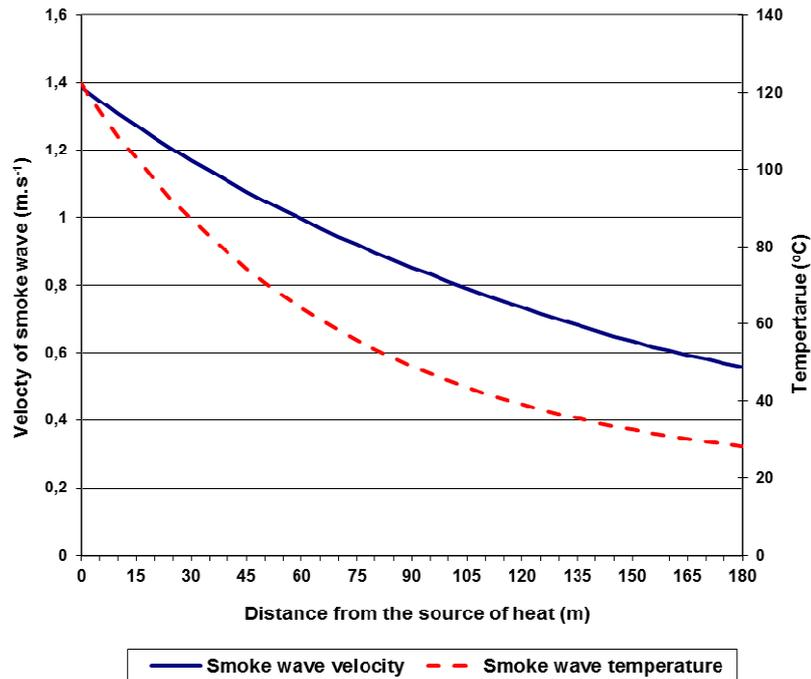
Fig. 3. Parameters of the smoke wave determined upon the input values of 2<sup>nd</sup> test [17].
