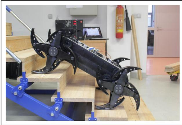
**Figure 19.** Mobile robot with the segmented wheels on stairs.
