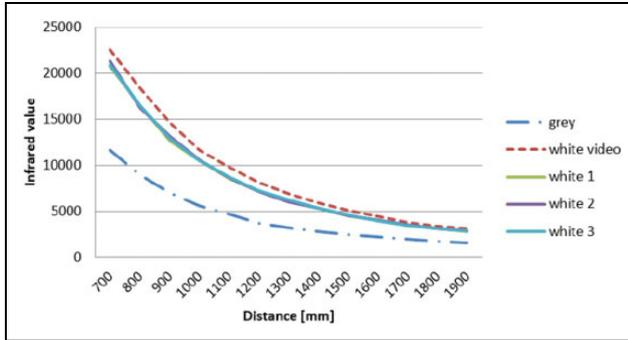
**Figure 3.** Course of IR value based on a distance and on captured surface color. IR: infrared.
