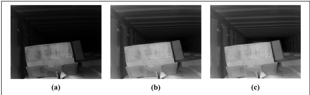
**Figure 9.** Infrared correction of the data set from a shipping container. (a) Default image, (b) gamma correction 0.5, and (c) correction by depth.
