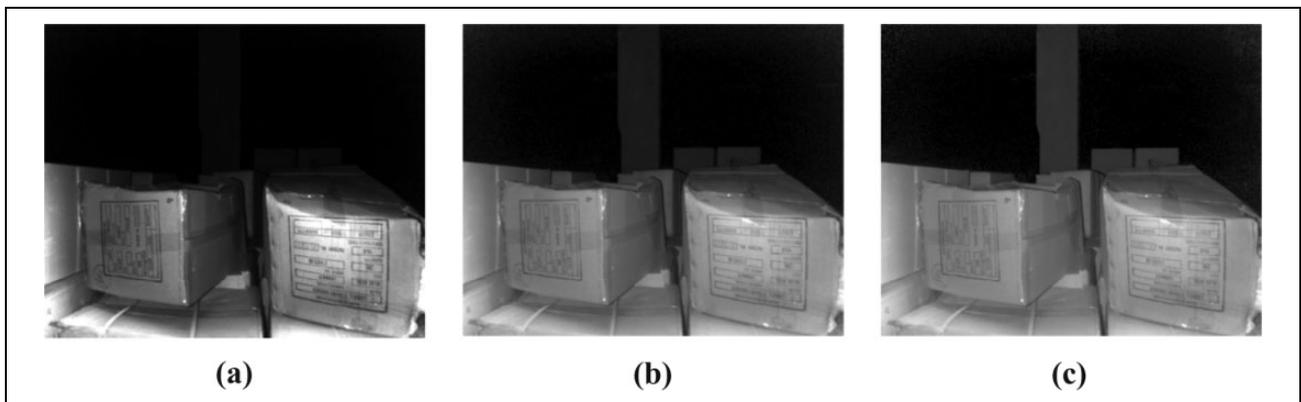
**Figure 10.** Infrared correction of the data set of cardboard boxes. (a) Default image, (b) gamma correction 0.5, and (c) correction by depth.
