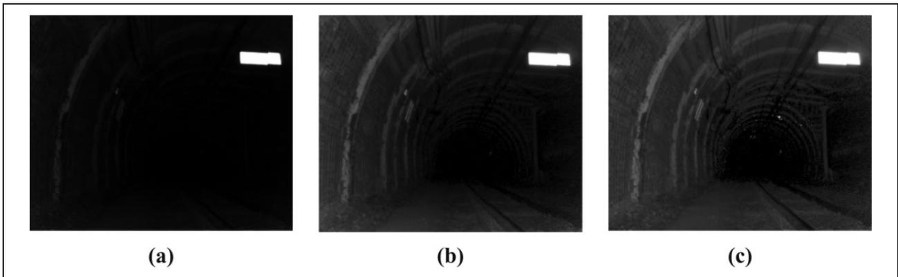
**Figure 8.** Infrared correction of the data set from a coal mine. (a) Default image, (b) gamma correction 0.5, and (c) correction by depth.
